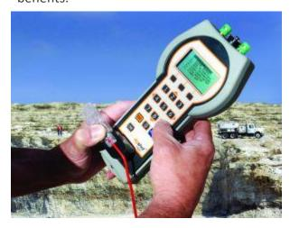
End-user training time is minimized with the easy-to-use menu-driven software and the hook-up process is quicker because pattern and delay timing can be entered ahead of time.
